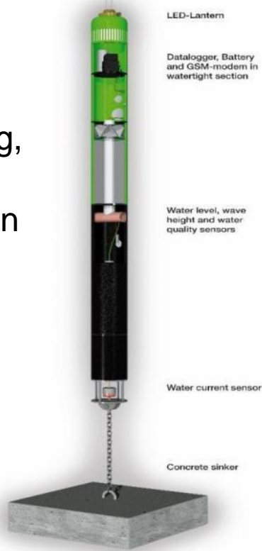
Schematic diagram of the SmartBuoy concept
